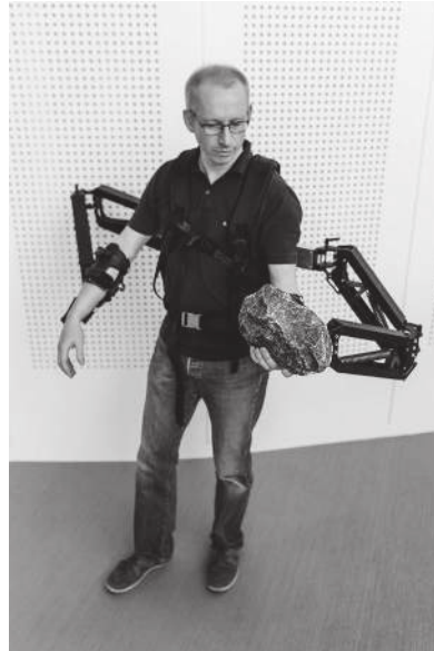
Figure 3: Prototype of Robo-Mate arm module
